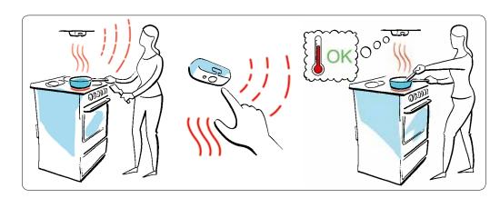
Pressing the Intelligent Heat Sensor cover during the pre-alarm signal • ) stops the alarm and the Stove Guard adjusts its sensitivity automatically.
