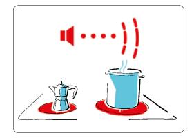
Using a pot much smaller than a hotplate can trigger an alarm.
