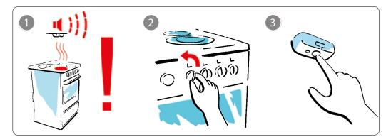
If the Stove Guard has turned the range off, first turn all range knobs off, then press the Heat Sensor cover once. (In ranges that are operated by touch, just press the Sensor cover once.) After this the range can be used normally.
